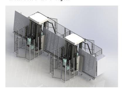
2 VX are installed in tandem with 3 conveyors between each laminator.
